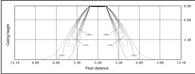
Figure 22. Cooling air velocity distribution: 4MUS4518**
